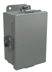
Wiegmann enclosure, NEMA 4/12/13, 6 x 4 x 3in (HxWxD), wall mount, carbon steel, ANSI 61 gray, powder coat finish, lift-off cover, (4) stainless steel clamps.
