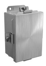
Wiegmann enclosure, NEMA 4/4X/12/13, 6 x 4 x 3in (HxWxD), wall mount, 304 stainless steel, No. 3 intermediate polished finish, lift-off cover, (4) stainless steel clamps.
