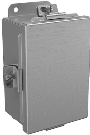
Wiegmann enclosure, NEMA 4/4X/12/13, 6 x 4 x 3in (HxWxD), wall mount, 5052-H32 aluminum, No. 3 intermediate polished finish, lift-off cover, (4) stainless steel clamps.
