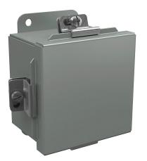
Wiegmann enclosure, NEMA 4/12/13,  $4 \times 4 \times 3$ in (HxWxD), wall mount, carbon steel, ANSI 61 gray, powder coat finish, lift-off cover, (4) stainless steel clamps.
