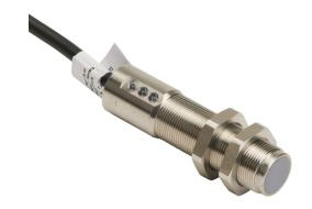
IDEM Z-Range safety switch set, non-contact uniquely coded RFID, (2) OSSD safety output(s), (1) status monitoring output(s), 316 stainless steel housing, 18mm diameter x 73mm body, 8-pin M12 quick-disconnect, 9.8in/250mm cable length.
