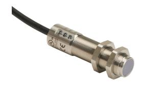
IDEM Z-Range safety switch set, non-contact uniquely coded RFID, (2) OSSD safety output(s), (1) status monitoring output(s), 316 stainless steel housing, 18mm diameter x 73mm body, pigtail, 32.8ft/10m cable length.
