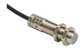
IDEM Z-Range safety switch set, non-contact uniquely coded RFID, (2) OSSD safety output(s), (1) status monitoring output(s), 316 stainless steel housing, 18mm diameter x 73mm body, pigtail, 16.4ft/5m cable length.
