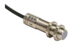
IDEM Z-Range safety switch set, non-contact master coded RFID, (2) OSSD safety output(s), (1) status monitoring output(s), 316 stainless steel housing, 18mm diameter x 73mm body, 8-pin M12 quick-disconnect, 9.8in/250mm cable length.
