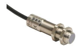
IDEM Z-Range safety switch set, non-contact master coded RFID, (2) OSSD safety output(s), (1) status monitoring output(s), 316 stainless steel housing, 18mm diameter x 73mm body, pigtail, 32.8ft/10m cable length.
