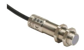
IDEM Z-Range safety switch set, non-contact master coded RFID, (2) OSSD safety output(s), (1) status monitoring output(s), 316 stainless steel housing, 18mm diameter x 73mm body, pigtail, 16.4ft/5m cable length.
