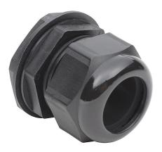
Bimed cable gland, PG36 thread type, polyamide, black, accepts 22 to 32mm diameter cable, IP68. Package of 2. Mounting hardware included.
