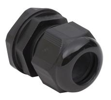
Bimed cable gland, PG21 thread type, polyamide, black, accepts 13 to 18mm diameter cable, IP68. Package of 5. Mounting hardware included.
