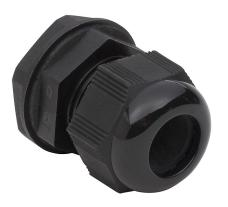
Bimed cable gland, PG16 thread type, polyamide, black, accepts 10 to 14mm diameter cable, IP68. Package of 5. Mounting hardware included.
