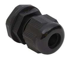
Bimed cable gland, PG11 thread type, polyamide, black, accepts 5 to 10mm diameter cable, IP68. Package of 5. Mounting hardware included.
