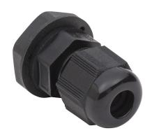
Bimed cable gland, PG7 thread type, polyamide, black, accepts 3 to 6.5mm diameter cable, IP68. Package of 5. Mounting hardware included.
