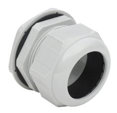
Bimed cable gland, PG48 thread type, polyamide, light gray, accepts 34 to 44mm diameter cable, IP68. Package of 2. Mounting hardware included.
