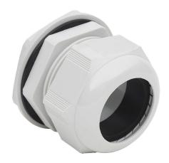
Bimed cable gland, PG42 thread type, polyamide, light gray, accepts 30 to 38mm diameter cable, IP68. Package of 2. Mounting hardware included.
