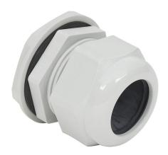
Bimed cable gland, PG36 thread type, polyamide, light gray, accepts 22 to 32mm diameter cable, IP68. Package of 2. Mounting hardware included.
