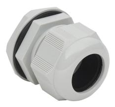
Bimed cable gland, PG29 thread type, polyamide, light gray, accepts 18 to 25mm diameter cable, IP68. Package of 5. Mounting hardware included.
