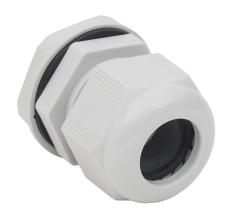
Bimed cable gland, PG21 thread type, polyamide, light gray, accepts 13 to 18mm diameter cable, IP68. Package of 5. Mounting hardware included.
