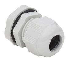
Bimed cable gland, PG13.5 thread type, polyamide, light gray, accepts 6 to 12mm diameter cable, IP68. Package of 5. Mounting hardware included.
