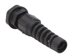
Bimed cable gland, M12 x 1.5mm thread type, polyamide, black, accepts 3 to 6.5mm diameter cable, IP68, with strain relief. Package of 5. Mounting hardware included.
