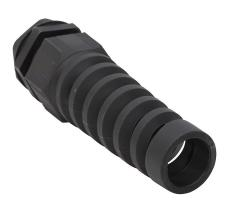
Bimed cable gland, M25 x 1.5mm thread type, polyamide, black, accepts 13 to 18mm diameter cable, IP68, with strain relief. Package of 5. Mounting hardware included.
