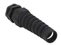
Bimed cable gland, M20 x 1.5mm thread type, polyamide, black, accepts 10 to 14mm diameter cable, IP68, with strain relief. Package of 5. Mounting hardware included.
