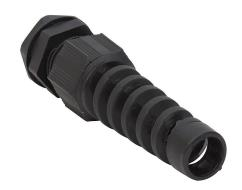
Bimed cable gland, M16 x 1.5mm thread type, polyamide, black, accepts 5 to 10mm diameter cable, IP68, with strain relief. Package of 5. Mounting hardware included.
