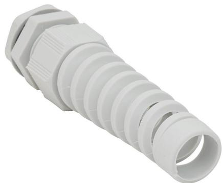
Bimed cable gland, M20 x 1.5mm thread type, polyamide, light gray, accepts 10 to 14mm diameter cable, IP68, with strain relief. Package of 5. Mounting hardware included.
