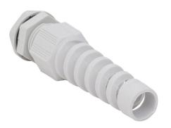
Bimed cable gland, M16 x 1.5mm thread type, polyamide, light gray, accepts 5 to 10mm diameter cable, IP68, with strain relief. Package of 5. Mounting hardware included.
