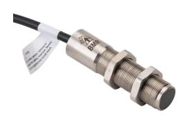
IDEM safety switch set, non-contact magnetic, (2) N.C. safety output(s), (1) N.O. monitoring output(s), 316 stainless steel housing, 18mm diameter x 75mm body, 8-pin M12 quick-disconnect, 9.8in/250mm cable length.
