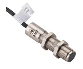
IDEM safety switch set, non-contact magnetic, (2) N.C. safety output(s), (1) N.O. monitoring output(s), 316 stainless steel housing, 18mm diameter x 75mm body, pigtail, 16.4ft/5m cable length.
