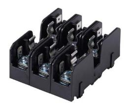
Bussmann modular fuse block, accepts Midget fuses, 30A, 600V, 3-pole, 18-10 AWG copper only, pressure plate with quick-connect terminals, 35mm DIN rail or panel mount. Package of 5.
