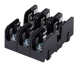
Bussmann modular fuse block, accepts Midget fuses, 30A, 600V, 3-pole, 18-10 AWG copper only, pressure plate with quick-connect terminals, 35mm DIN rail or panel mount. Package of 5.
