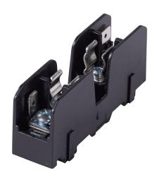
Bussmann modular fuse block, accepts Midget fuses, 30A, 600V, 1-pole, 18-10 AWG copper only, pressure plate with quick-connect terminals, 35mm DIN rail or panel mount. Package of 15.
