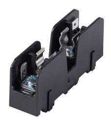
Bussmann modular fuse block, accepts Midget fuses, 30A, 600V, 1-pole, 18-10 AWG copper only, pressure plate with quick-connect terminals, 35mm DIN rail or panel mount.
