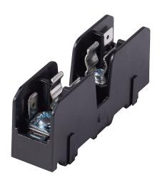
Bussmann modular fuse block, accepts Midget fuses, 30A, 600V, 1-pole, 18-10 AWG copper only, pressure plate with quick-connect terminals, 35mm DIN rail or panel mount.
