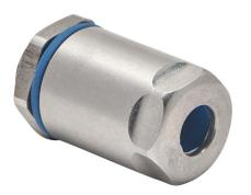
Bimed hygienic cable gland, M12 x 1.5mm thread type, stainless steel, accepts 3 to 6.5mm diameter cable, IP66, IP68 and IP69. Mounting hardware included. Allen wrench size 7mm, use adapter BMFGT-01 to reduce Allen wrench size to 5mm.
