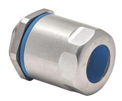
Bimed hygienic cable gland, M25 x 1.5mm thread type, stainless steel, accepts 12 to 17mm diameter cable, IP66, IP68 and IP69. Mounting hardware included. Allen wrench size 17mm, use adapter BMFGT-04 to reduce Allen wrench size to 10mm.
