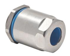
Bimed hygienic cable gland, M20 x 1.5mm thread type, stainless steel, accepts 6 to 12mm diameter cable, IP66, IP68 and IP69. Mounting hardware included. Allen wrench size 13mm, use adapter BMFGT-03 to reduce Allen wrench size to 8mm.
