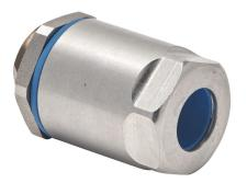
Bimed hygienic cable gland, M16 x 1.5mm thread type, stainless steel, accepts 5 to 10mm diameter cable, IP66, IP68 and IP69. Mounting hardware included. Allen wrench size 10mm, use adapter BMFGT-02 to reduce Allen wrench size to 6mm.
