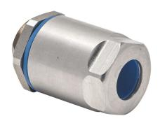
Bimed hygienic cable gland, M16 x 1.5mm thread type, stainless steel, accepts 5 to 10mm diameter cable, IP66, IP68 and IP69. Mounting hardware included. Allen wrench size 10mm, use adapter BMFGT-02 to reduce Allen wrench size to 6mm.
