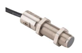
IDEM safety switch set, non-contact uniquely coded RFID, (2) N.C. safety output(s), (1) N.O. monitoring output(s), 316 stainless steel housing, 18mm diameter x 75mm body, 8-pin M12 quick-disconnect, 9.8in/250mm cable length.
