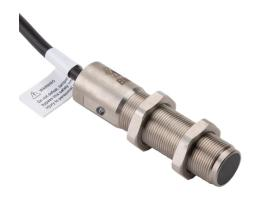
IDEM safety switch set, non-contact uniquely coded RFID, (2) N.C. safety output(s), (1) N.O. monitoring output(s), 316 stainless steel housing, 18mm diameter x 75mm body, pigtail, 32.8ft/10m cable length.
