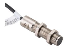
IDEM safety switch set, non-contact uniquely coded RFID, (2) N.C. safety output(s), (1) N.O. monitoring output(s), 316 stainless steel housing, 18mm diameter x 75mm body, pigtail, 16.4ft/5m cable length.
