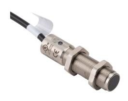
IDEM safety switch set, non-contact master coded RFID, (2) N.C. safety output(s), (1) N.O. monitoring output(s), 316 stainless steel housing, 18mm diameter x 75mm body, 8-pin M12 quick-disconnect, 9.8in/250mm cable length.
