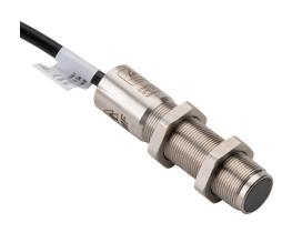
IDEM safety switch set, non-contact master coded RFID, (2) N.C. safety output(s), (1) N.O. monitoring output(s), 316 stainless steel housing, 18mm diameter x 75mm body, pigtail, 32.8ft/10m cable length.
