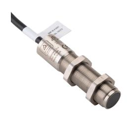
IDEM safety switch set, non-contact master coded RFID, (2) N.C. safety output(s), (1) N.O. monitoring output(s), 316 stainless steel housing, 18mm diameter x 75mm body, pigtail, 16.4ft/5m cable length.
