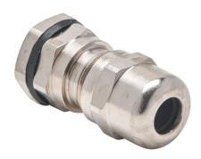
Bimed EMC cable gland, M12 x 1.5mm thread type, nickel-plated brass, accepts 3 to 6.5mm diameter cable, IP68. Package of 5. Mounting hardware included.
