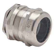
Bimed EMC cable gland, M63 x 1.5mm thread type, nickel-plated brass, accepts 37 to 53mm diameter cable, IP68. Package of 2. Mounting hardware included.
