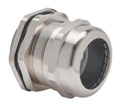
Bimed EMC cable gland, M63 x 1.5mm thread type, nickel-plated brass, accepts 34 to 44mm diameter cable, IP68. Package of 2. Mounting hardware included.
