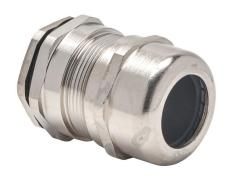
Bimed EMC cable gland, M32 x 1.5mm thread type, nickel-plated brass, accepts 16 to 25mm diameter cable, IP68. Package of 5. Mounting hardware included.
