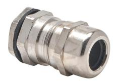
Bimed EMC cable gland, M20 x 1.5mm thread type, nickel-plated brass, accepts 7.5 to 14mm diameter cable, IP68. Package of 5. Mounting hardware included.
