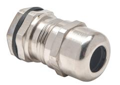
Bimed EMC cable gland, M16 x 1.5mm thread type, nickel-plated brass, accepts 5 to 10mm diameter cable, IP68. Package of 5. Mounting hardware included.
