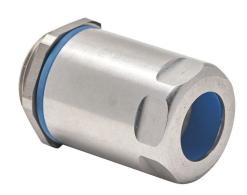
Bimed hygienic EMC cable gland, M25 x 1.5mm thread type, stainless steel, accepts 12 to 17mm diameter cable, IP66, IP68 and IP69. Mounting hardware included. Allen wrench size 17mm, use adapter BMFGT-04 to reduce Allen wrench size to 10mm.
