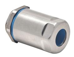
Bimed hygienic EMC cable gland, M20 x 1.5mm thread type, stainless steel, accepts 6 to 12mm diameter cable, IP66, IP68 and IP69. Mounting hardware included. Allen wrench size 13mm, use adapter BMFGT-03 to reduce Allen wrench size to 8mm.
